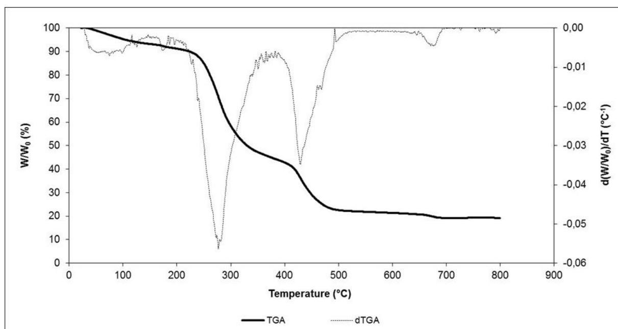
**Figure 1** Plot of percentage of residual sample weight, relative to starting sample weight ( $W/W_0$ , %), and first derivative  $d(W/W_0)/dT$ , versus temperature ( $T$ , °C). Data for raw 5-10 mm post-harvest tomato plant powder (PHTr).
